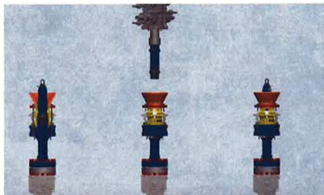
Figure 4. RigLock Allows PCE To Be Detached/Stubbed & Locked Quickly By Crane/Remote Switch
